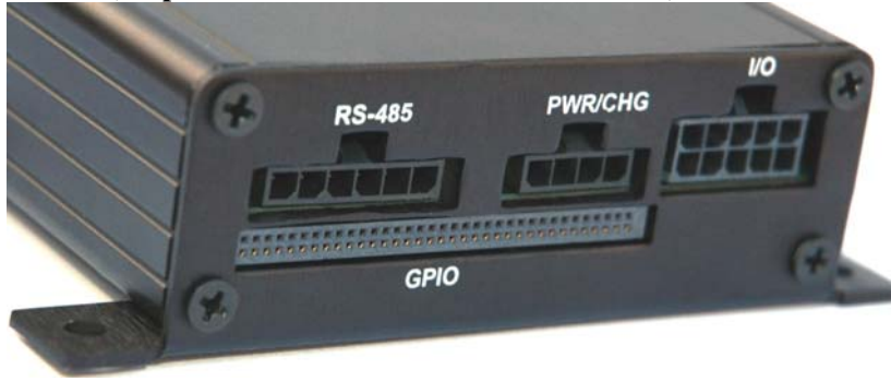
Figure 1.2.3.2: Modem Rear Panel Interface (All possible connections shown for reference)
